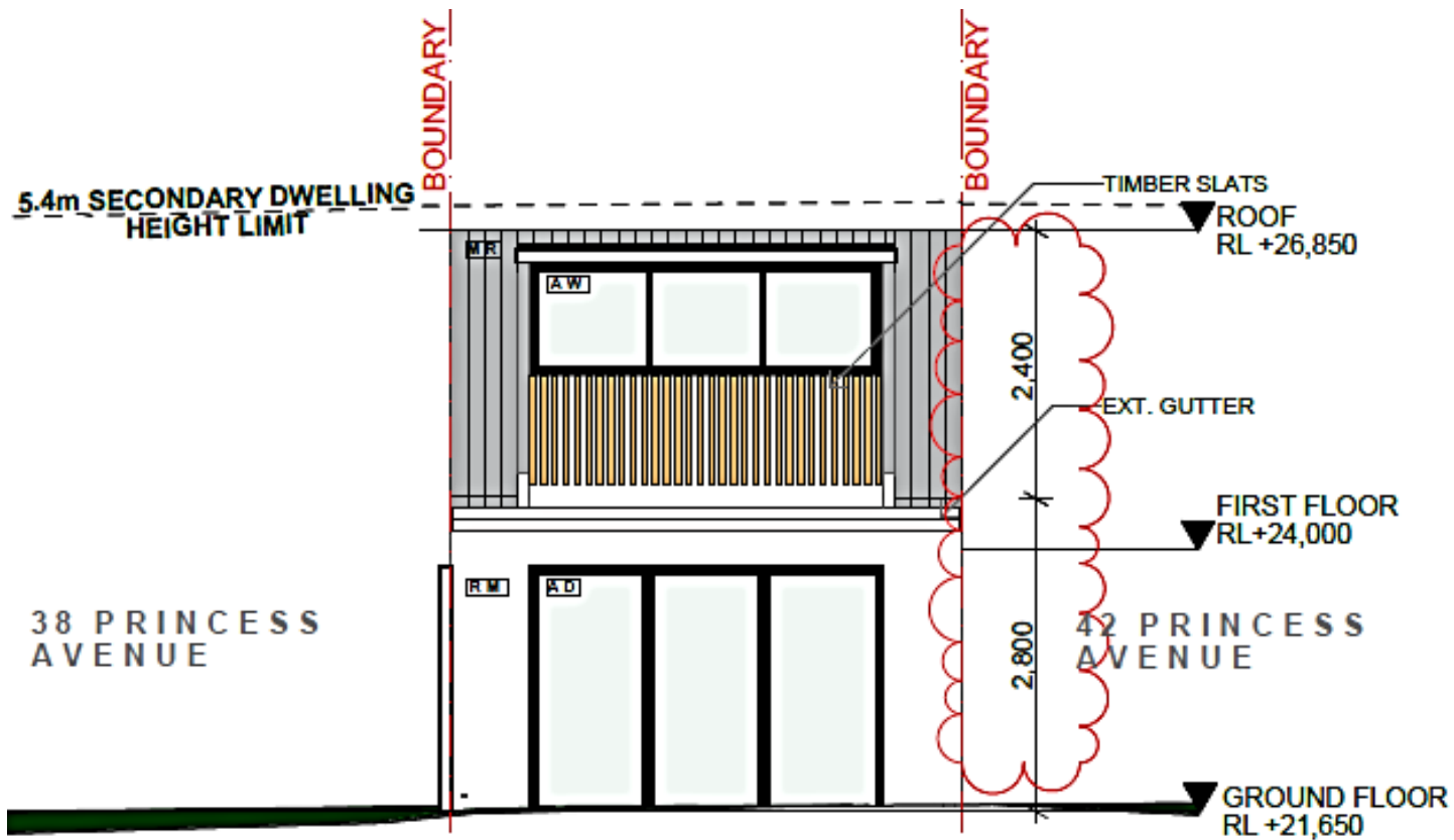
internal rear yard elevation
